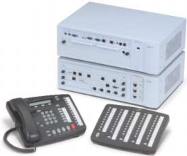
3Com SuperStack 3 NBX Networked Telephony Solution with the NBX V5000 chassis/call processor stack, Business Phone, and Attendant Console.
