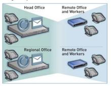
Note: VCX Connect 100 system configurations are shown above. VCX Connect 200 systems can support the same server configurations, but require separate gateways at head and regional offices.
