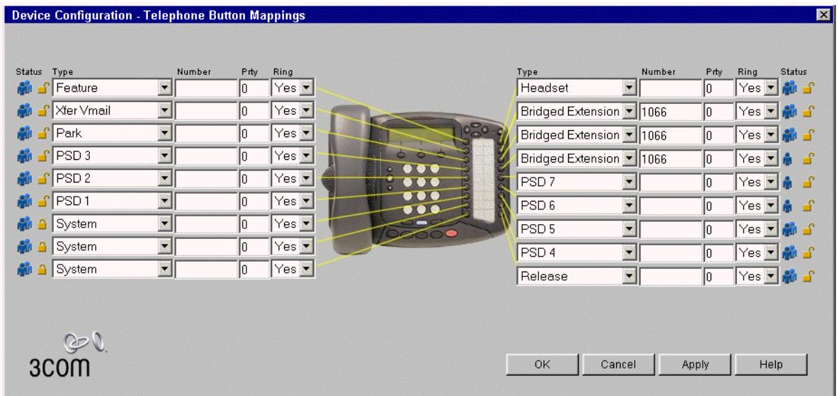
[Figure 20](#) shows a group of three buttons that have been configured as bridged extension appearances for the extension (1066) associated with the primary telephone.
