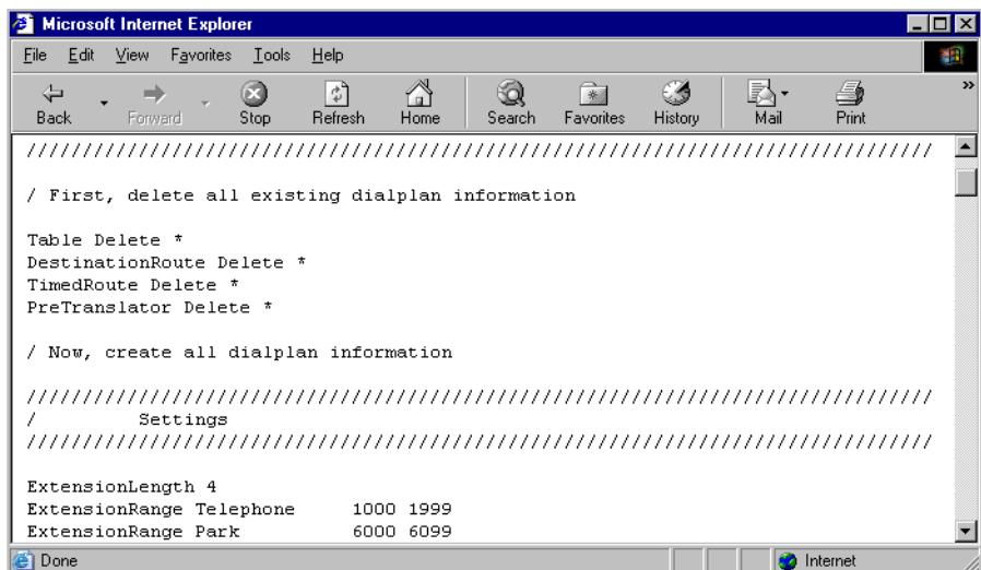
The screenshot shows a Microsoft Internet Explorer window displaying a text-based dial plan configuration file. The file contains comments and several configuration entries. The configuration includes deleting existing dialplan information and creating new settings, such as extension ranges for telephone numbers.
