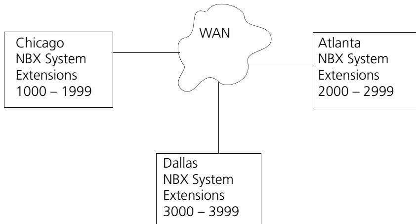
In the sample network shown in [Figure 10](#), each site is set up to use a unique range of telephone extensions. The dial plan on each of the systems is configured so that whenever a call is made to an extension not located at the local site, the NBX system sets up a VTL connection to the appropriate site.
