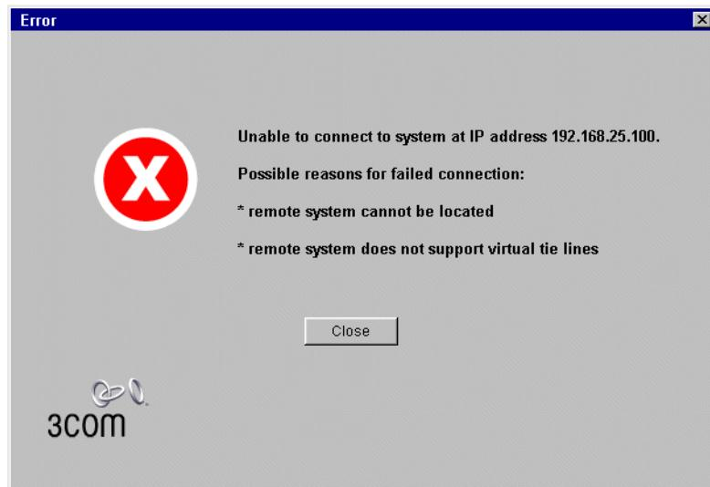
If you have not yet configured the remote system to support VTLs, this message indicates that you must do so before the Query Remote operation can succeed.
